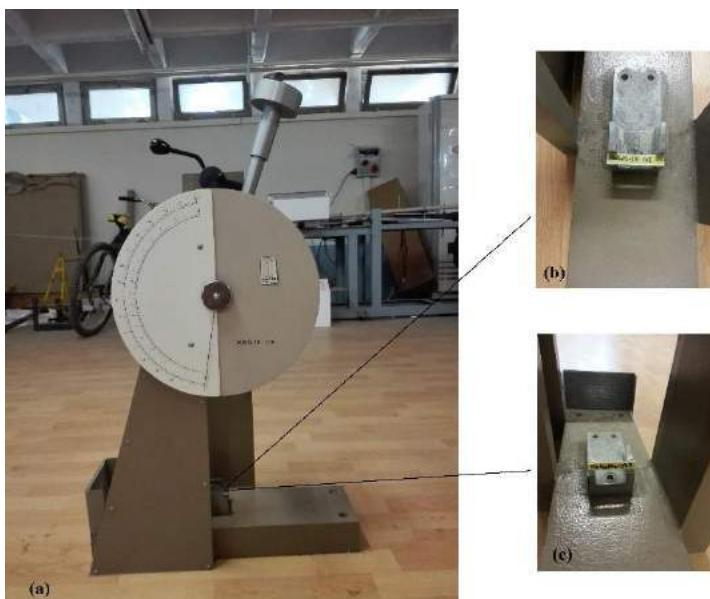
**Figure 2. Charpy Impact Test Machine Type Köger 3/70; a) Test Device, b) Notched Sample for Edgewise Impact, c) Un-notched Sample for Flatwise Impact**
