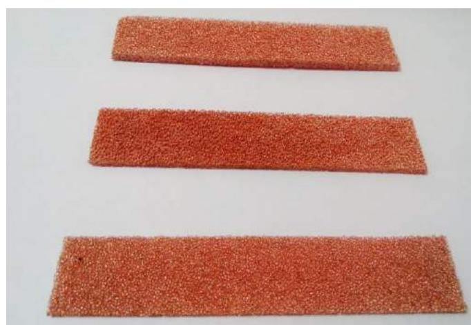
**Figure 2. Plate Type Copper Foam Test Samples**
