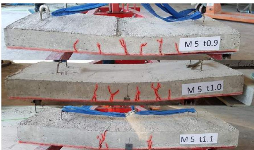
**Figure 34. Cracks Pattern Of M5 Groups**
