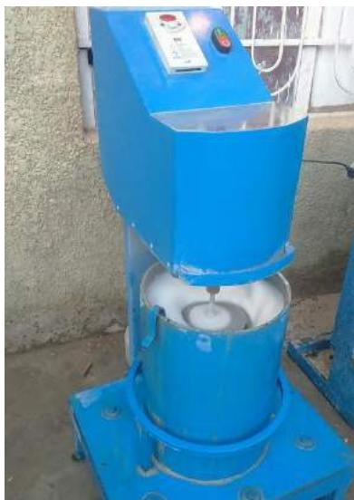
**Figure 3. The Used ASTM C1138 Testing Machine during Testing**
