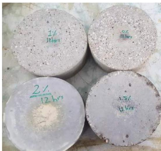
Figure 4. The Cylindrical Test Specimens after 12 Hours of Abrasion Test
