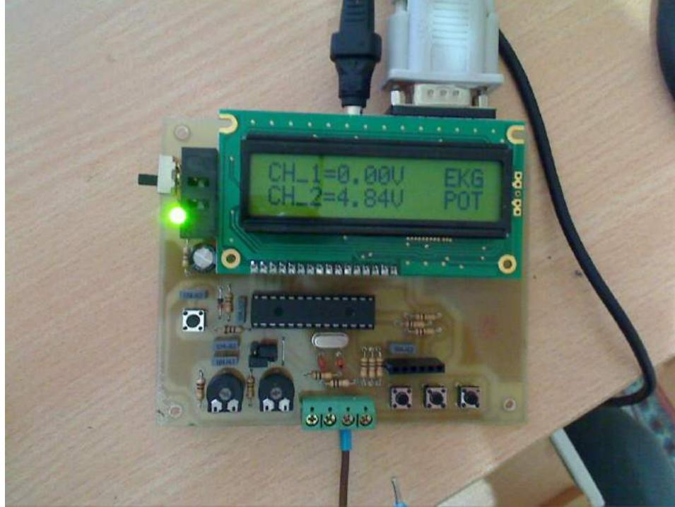
Fig.6 PIC 16F876A analog to digital conversion board with the RS232 module
