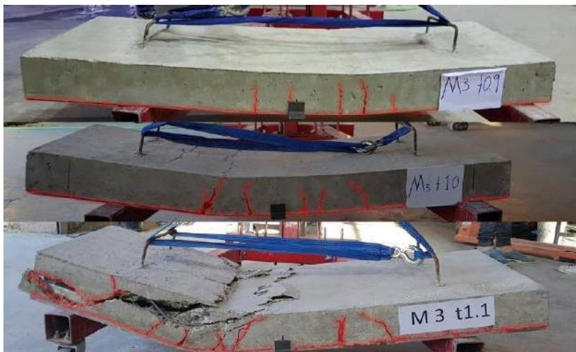
**Figure 32. Cracks Pattern Of M3 Groups**
