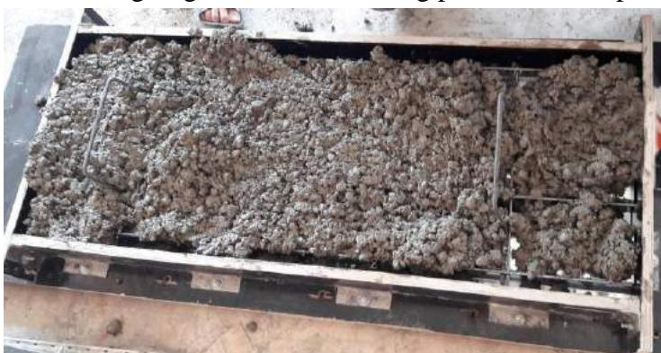
**Figure 10. Casting Process Of The Slab Specimens**
