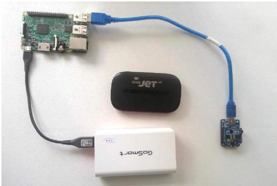
**Figure 1: Central Control Unit using Raspberry Pi-3**
