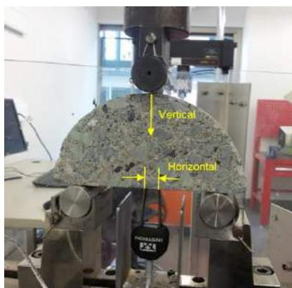
**Figure 4. SCB Testing Setup**
