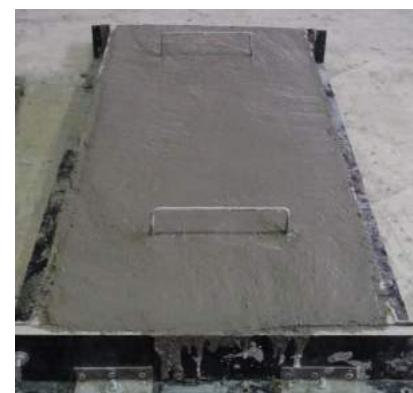
**Figure 11. The Composite Slab Specimen After Casting**
