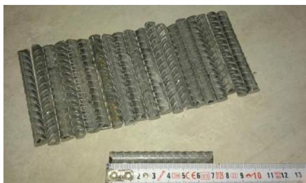
Figure 7. The Shear Connectors Used In The Present Study
