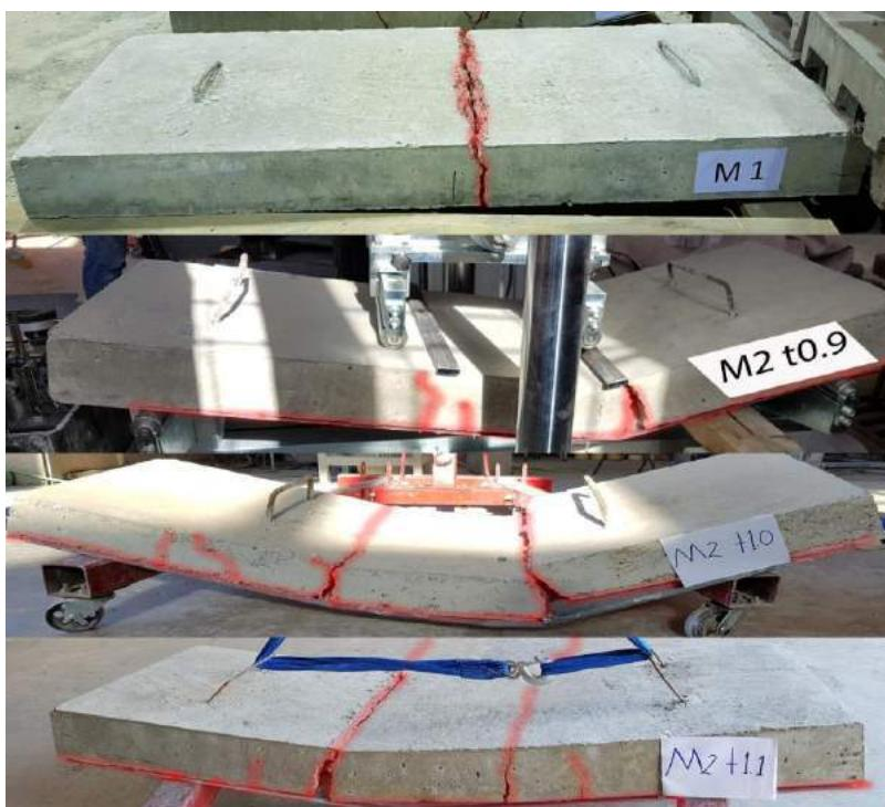
**Figure 31. Cracks Pattern Of M1 And M2 Groups**
