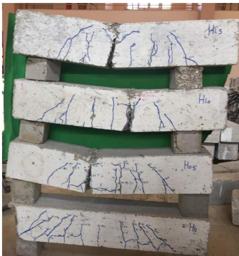
**Figure 8. Cracks Patterns of tested beams**
