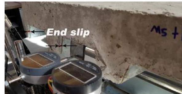
**Figure 19. Slip At The Right End Of M5 t1.0 Specimen.**
