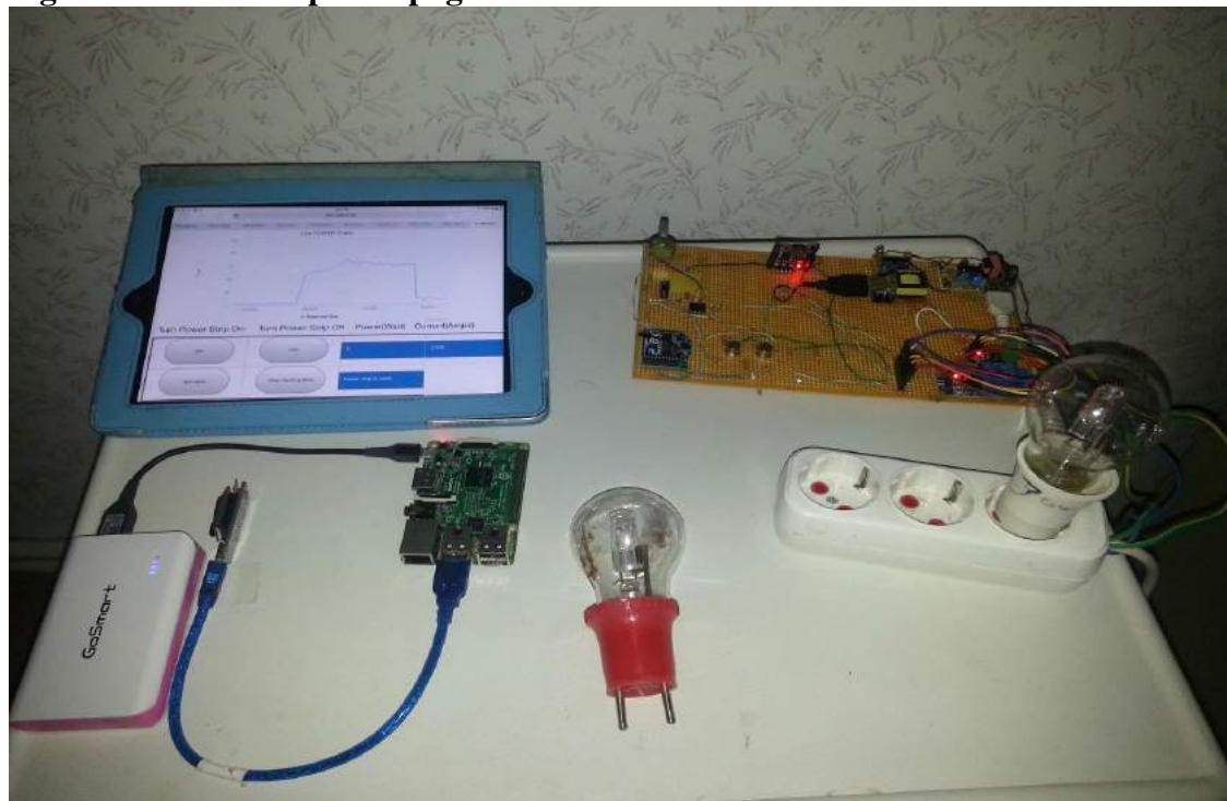
Figure 4: Controlling the bulb by using tablet
