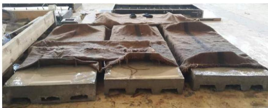
**Figure 12. Curing Process Of The Specimens**
