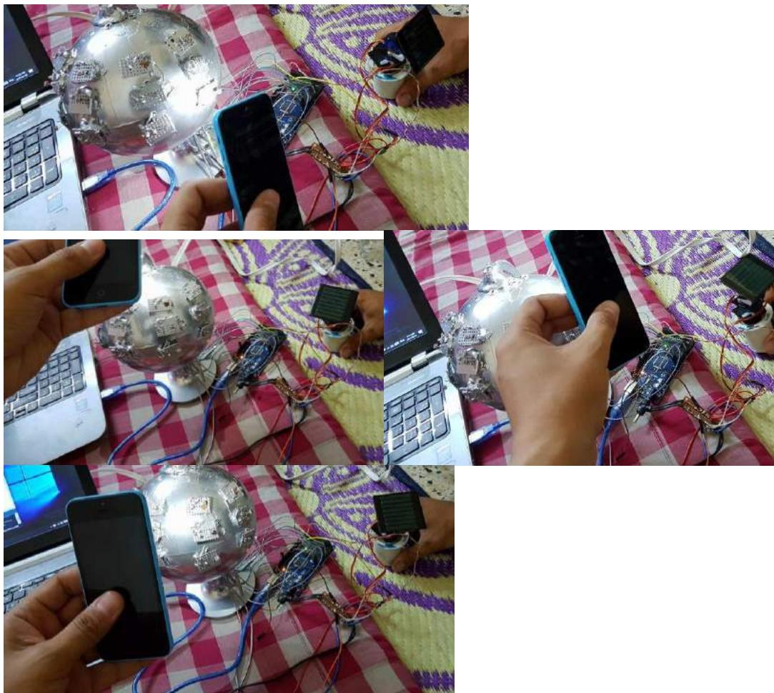
**Figure 4. Solar trucking system on work for different positions. The solar panel tracked the smartphone light that falls on power analyzer**
