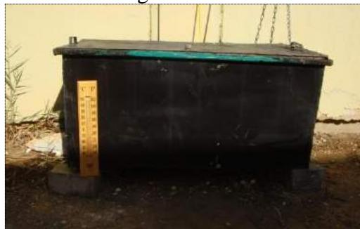
**Figure 2. Steam Curing Chamber**
