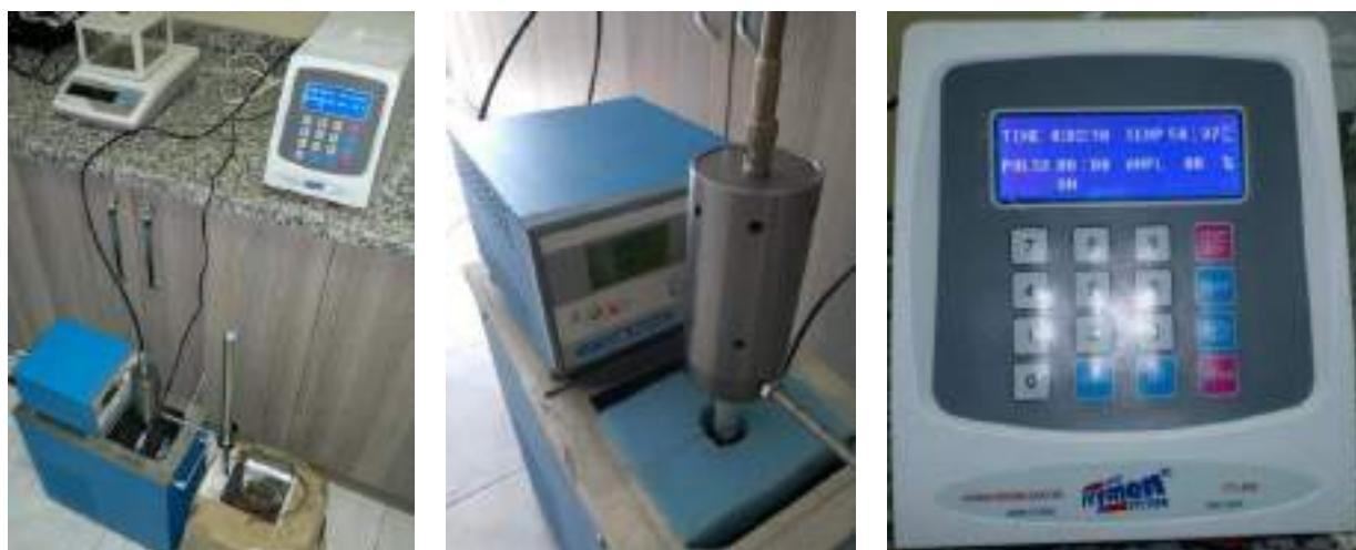
**Figure 1.** Preparation of nanofluid with temperature control
