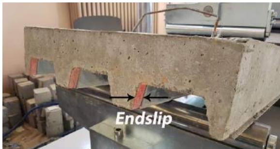
**Figure 18. Slip At The Left End Of M2 t1.0 Specimen**
