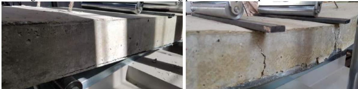
**Figure 29. De-lamination Of Concrete And Profiled Steel Sheeting Along The Length Of The Slab**
