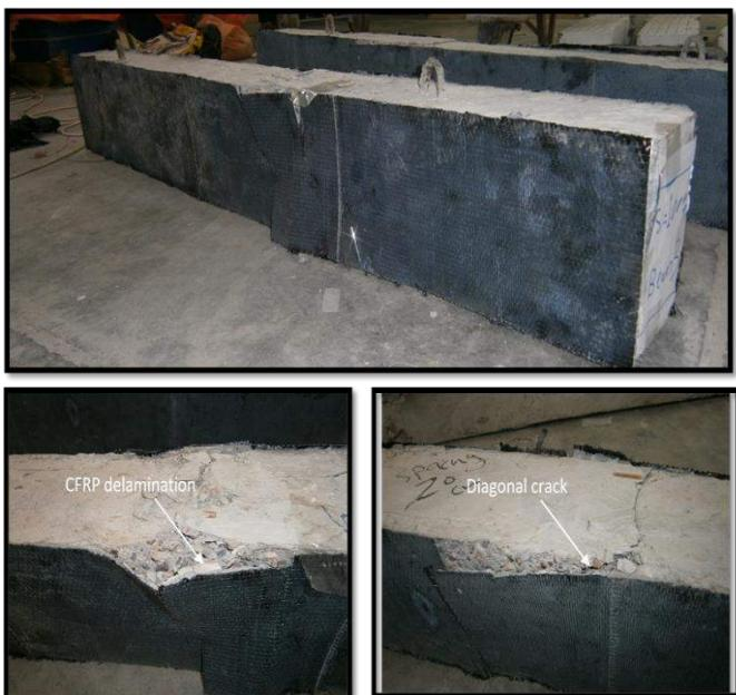
**Figure 4. Failure Mode**
