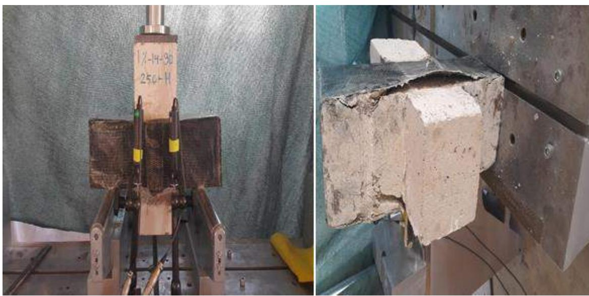
**Figure 5.** Specimen with De-bonding failure
